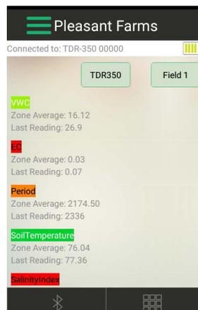
Figure 7b - Grid Mode Readings Screen
